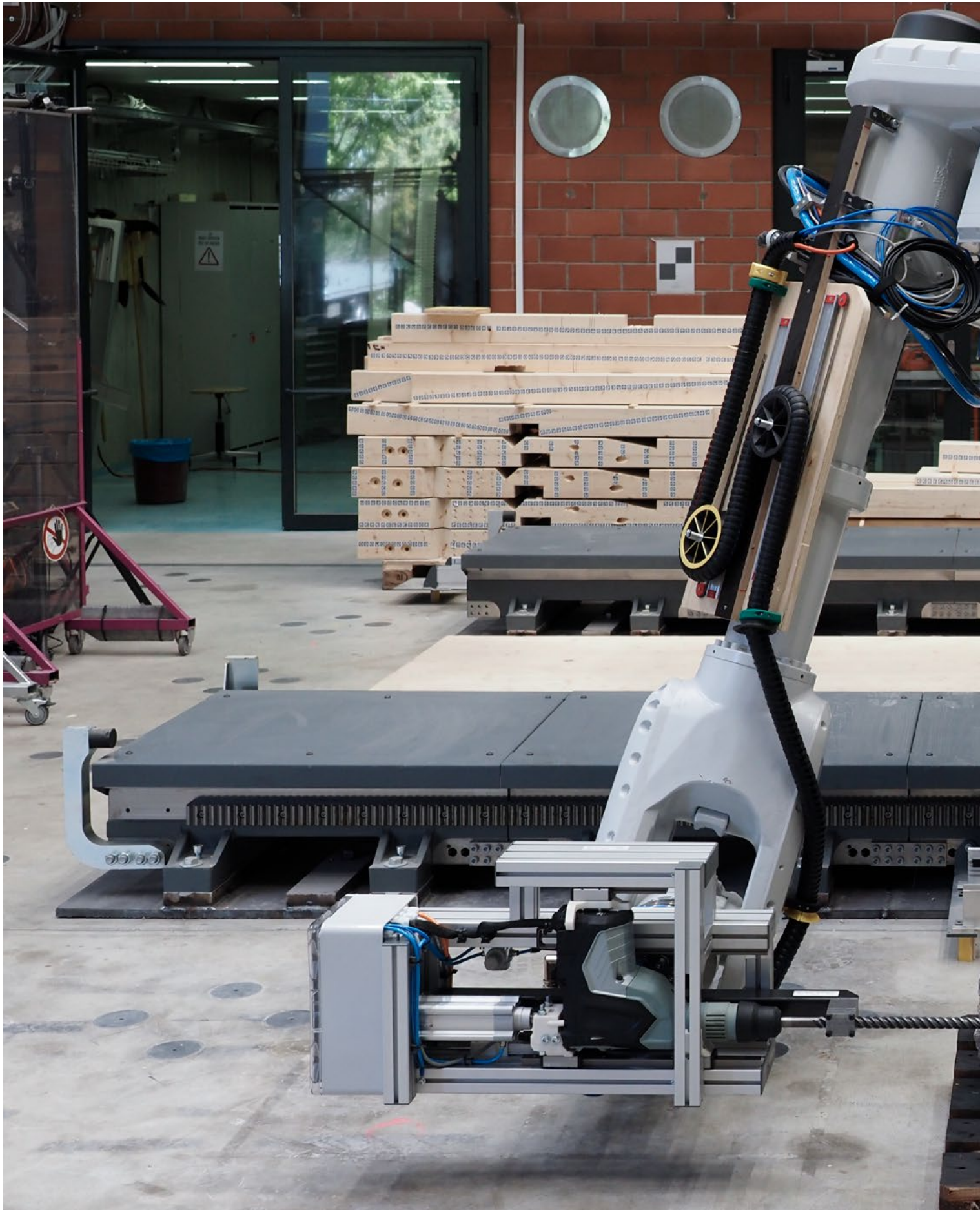
Robotic drilling of large concrete rubble, SXL, Structural Exploration Lab and CRCL, Lab for Creative Computation, EPFL, 2023 Photo: Maxence Grangeot
